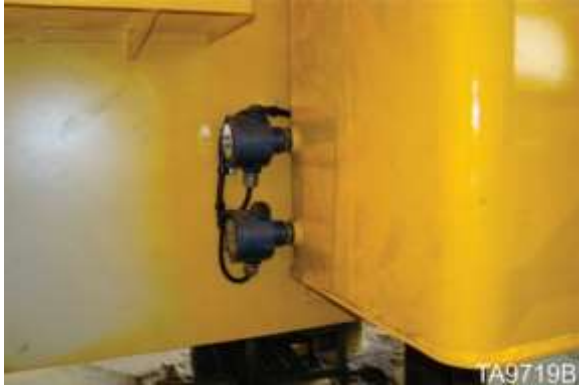
Heating elements are mounted inside of hydraulic reservoir
