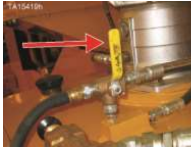
Figure 10. Hydraulic reservoir air valve handle UP
