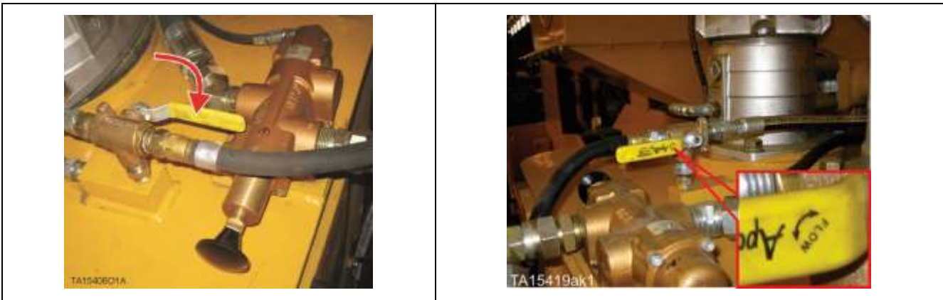
Figure 5. Air bleed valve in pressurized position (reservoir pressurized)
