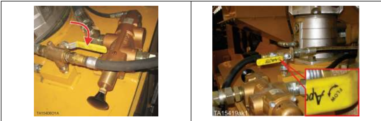
Figure 31. Air bleed valve in pressurized position (reservoir pressurized)
