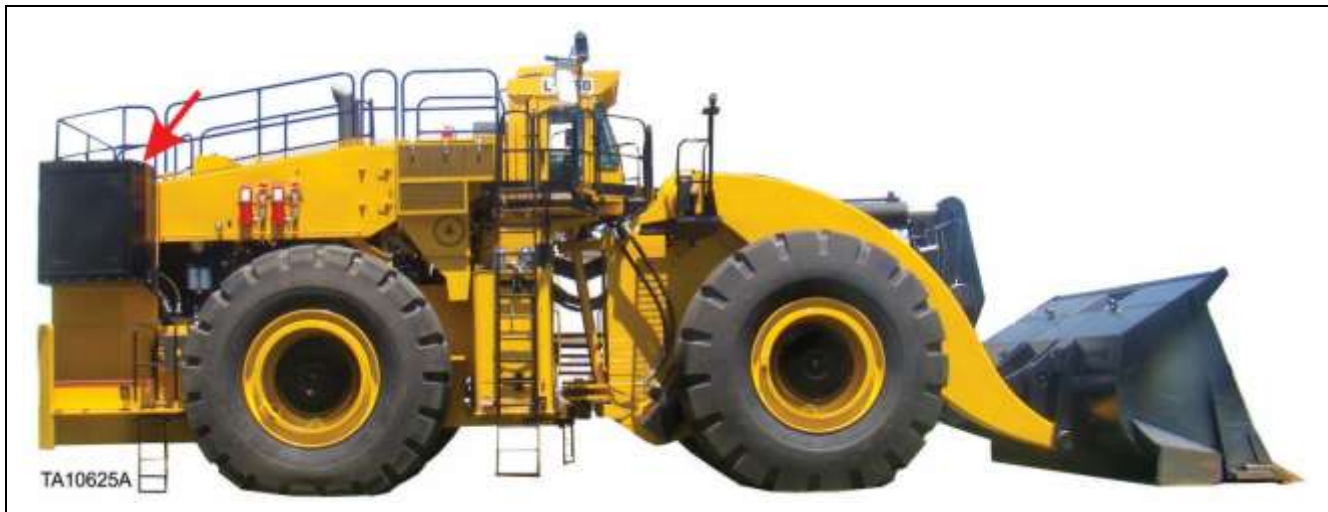
Figure 82. Auxiliary oil cooler typical location
