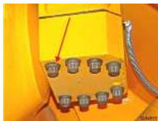
Arrow indicates location to be cleaned
