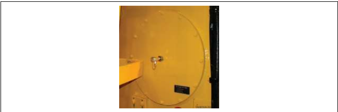
Figure 19. Hydraulic oil sampling quick connect fitting
