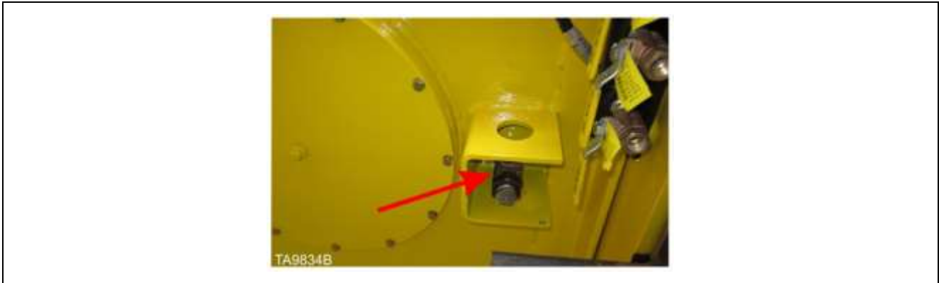
Figure 7. Hydraulic reservoir drain valve
