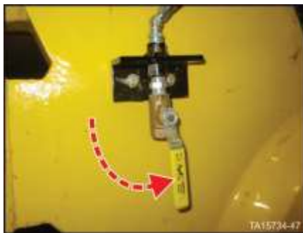
Figure 11. Air reservoir bleed valves in open position
